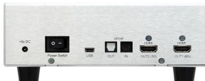
Figure 1.3. SL-881 AVG – Rear Panel
